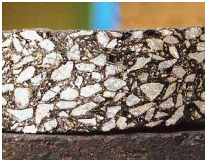
Figure 4-4. Stone-on-Stone Structure of SMA Mixture
