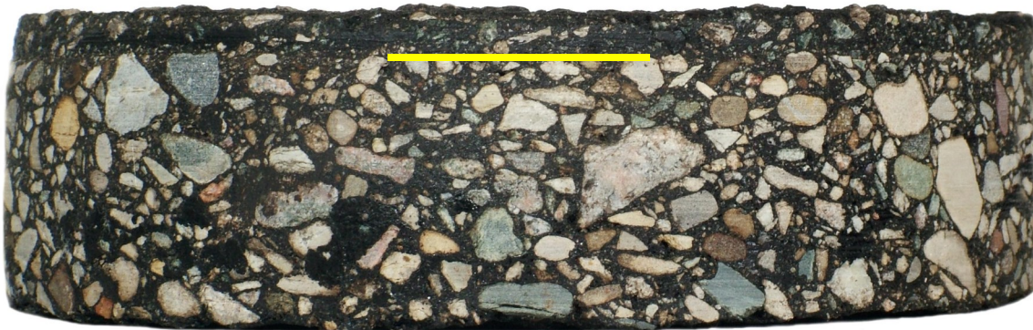
Typical Surface Treatment 3/16" - 3/8" Over existing asphalt pavement
