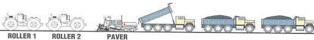
Delivery vehicle to paver direct method of paving. Causes segregation both of aggregate and temperature of paving material
