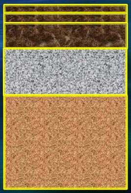
2" Gap-Graded Superpave Top 2.5" 4E30 Level
