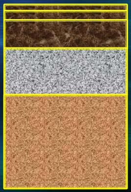
1.5" Gap-Graded Superpave Top 2.5" 4E30 Level
