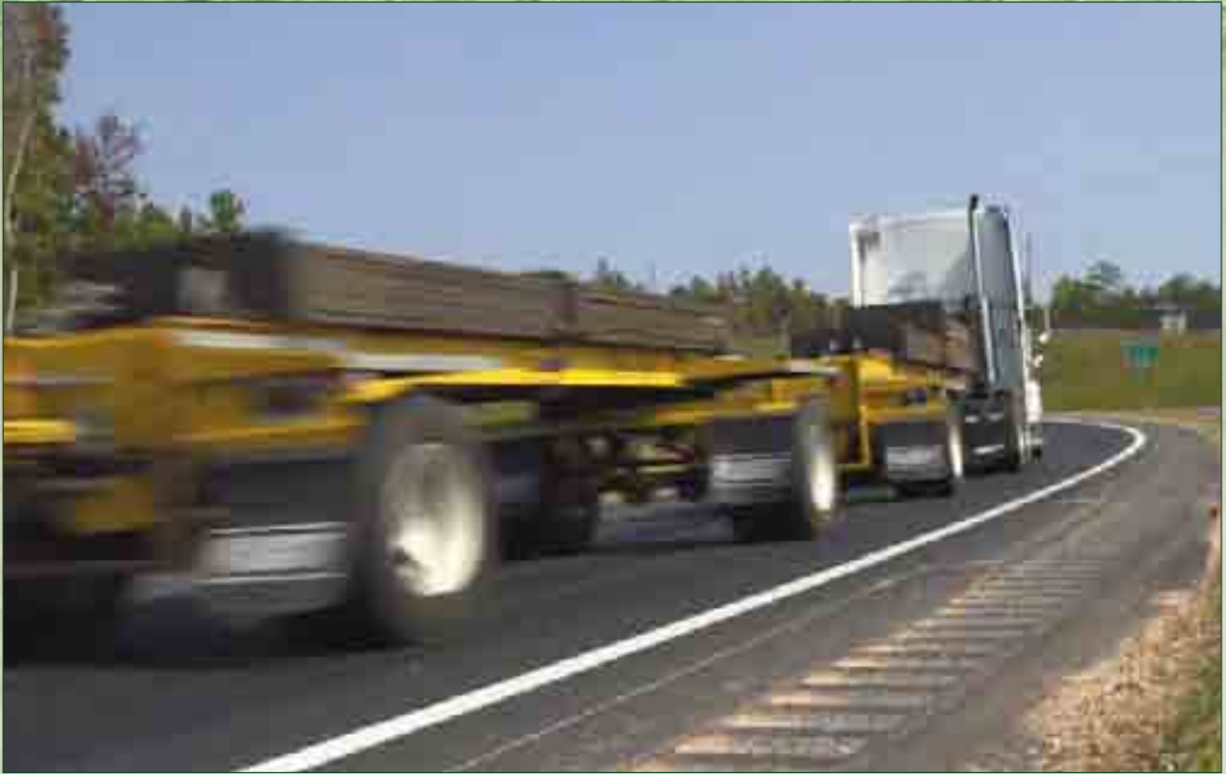
Research at the National Center for Asphalt Technology (NCAT) in Auburn, Alabama has showed that heavily loaded trucks driven on rough pavements consume more fuel than the same trucks driven on smooth pavements.
