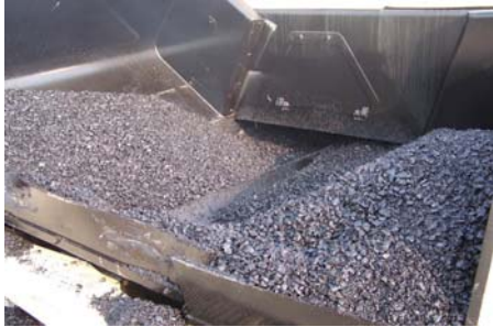
Conveyor area is exposed and augers are starved!
