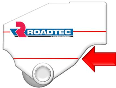
Make sure that the C2 has at least 1/3<sup>rd</sup> to 2/3<sup>rd</sup> capacity at all times.
