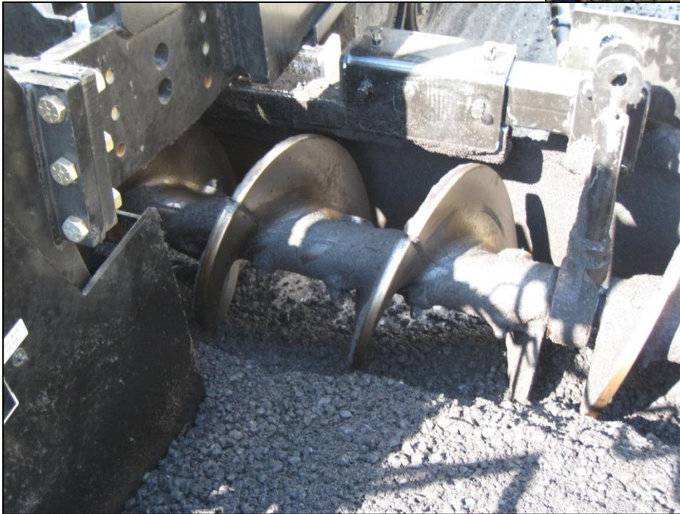
Improper operation of a paver can cause segregation in varying degrees.
