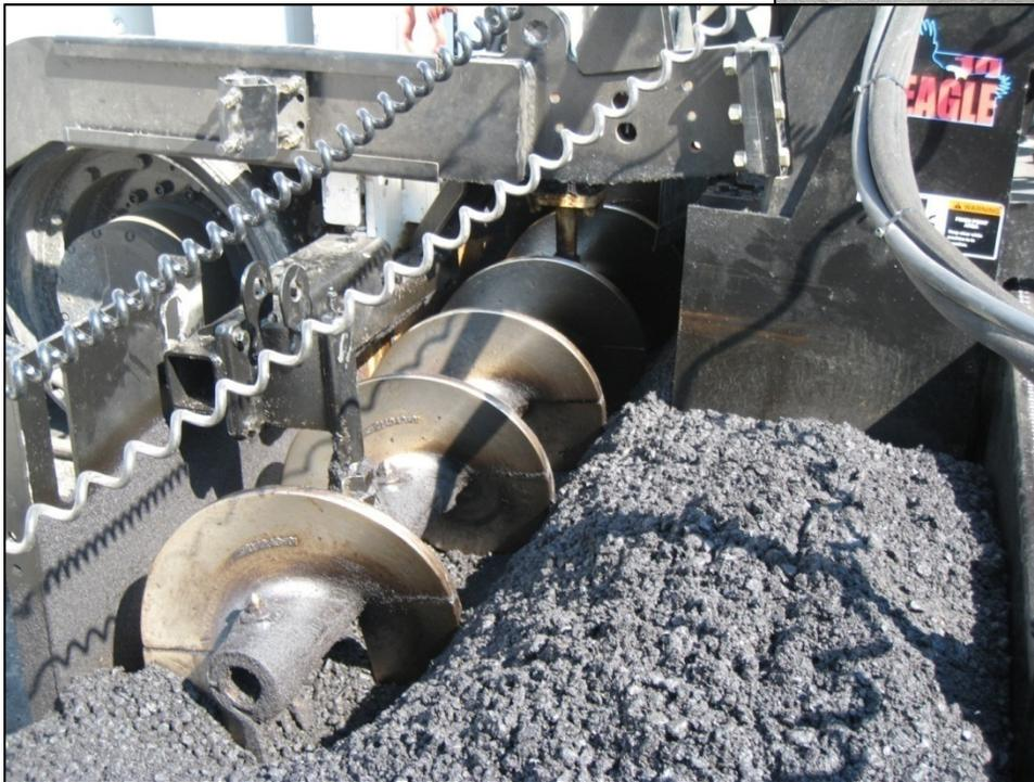
By starving the augers for mix, fine material will drop directly on the ground causing coarse material to be augered to each side.
