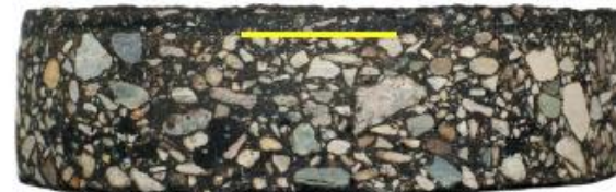
Typical Surface Treatment 3/16" - 3/8" Over existing asphalt pavement
